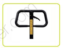
Manually operated brake. The pallet truck brake acts by means of two drum brakes on the directional wheels which can be in rubber or polyurethane and can be activated using the dedicated lever on the drawbar. It guarantees a stable and movement-free positioning of the pallet truck during parking
