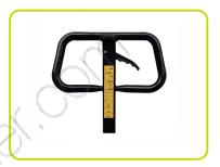
Manually operated brake. The pallet truck brake acts by means of two drum brakes on the directional wheels which can be in rubber or polyurethane and can be activated using the dedicated lever on the drawbar. It guarantees a stable and movement-free positioning of the pallet truck during parking
